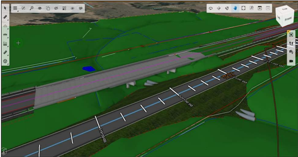
Figure 6 – OpenRoads and Open Bridge models displayed in Bentley Infrastructure Cloud
